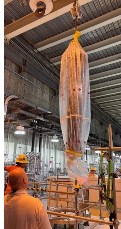
Sleeved Filter Upon Removal
